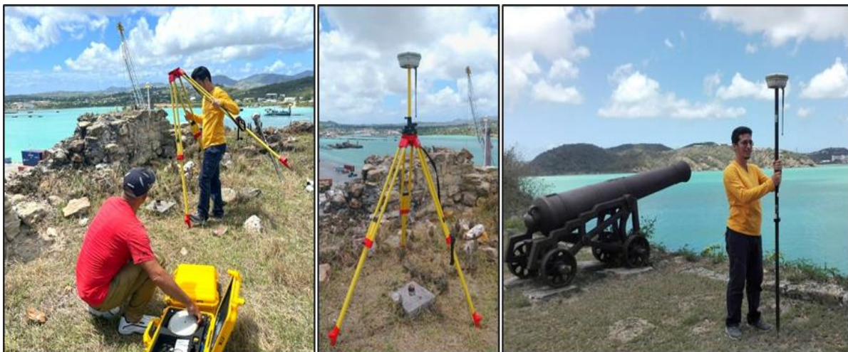
Frame 2: Survey of control points from the topographic benchmark in Rat Island, with coordinates provided by the Focal Point, using a high-precision geopositioning system (GPS) with real-time kinematic technology (RTK).
