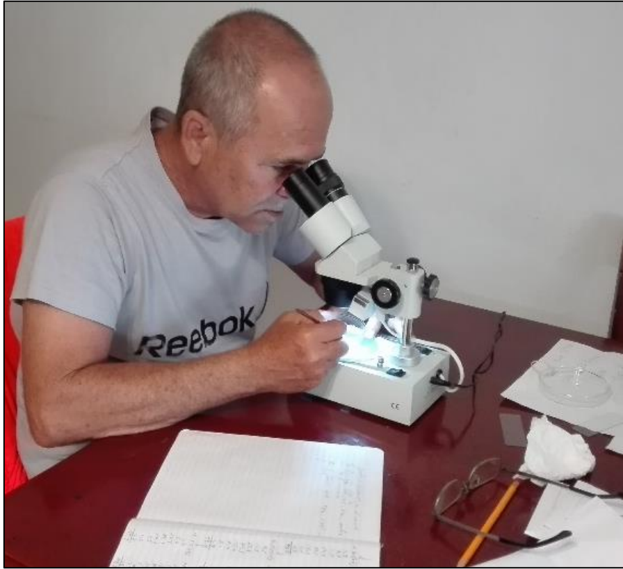
Photo 5: Analysis of sand samples under the microscope in the field laboratory. Grain size and composition analyses were performed on sand samples from Runaway Bay and the proposed borrow area.
