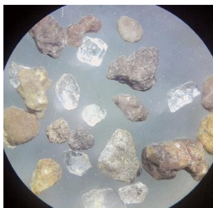
Photo 17: Grains of inorganic sand under the microscope. Sample taken at Runaway Bay. Tiny grains of quartzite, and even ferrous materials, from abrasion of adjacent cliff and rocky ledges.
