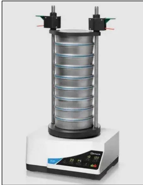
Photo 4: Sand samples were sifted for grain size analysis using a set of sieves belonging to the Retsh As 200 electronic sieve shaker.
