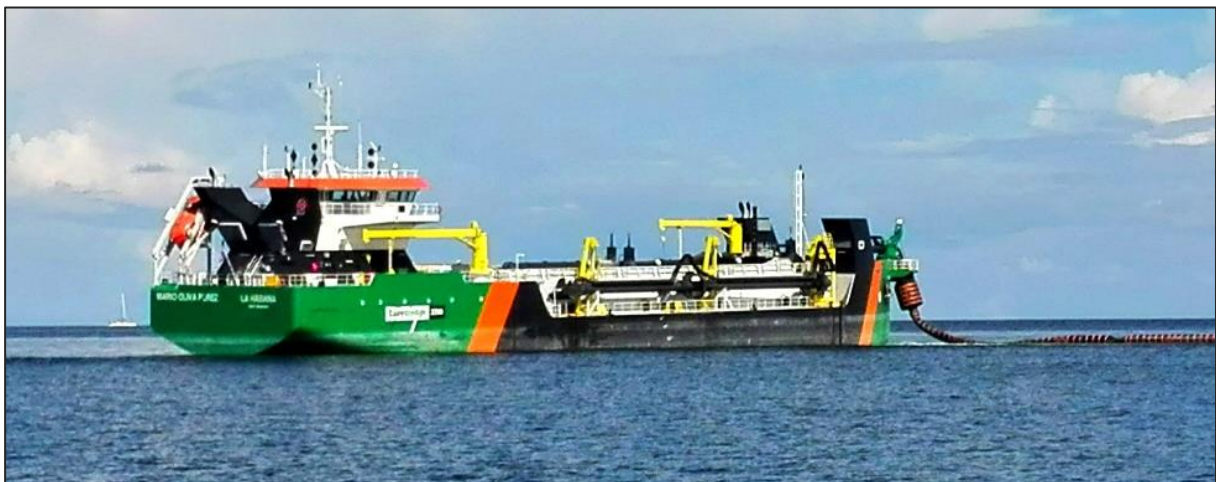
Photo 18: Example of a dredger with characteristics suitable for the execution of this project: Mario Oliva Pérez dredger (Building Company of Maritime Works, Cuba); length 92.95 m, beam 16.5 m, 3,300 m 3 hopper capacity, 6.20 m maximum draft, and power to pump a mixture of 1,280 kg/m 3 up at a distance of 4,500 m.
