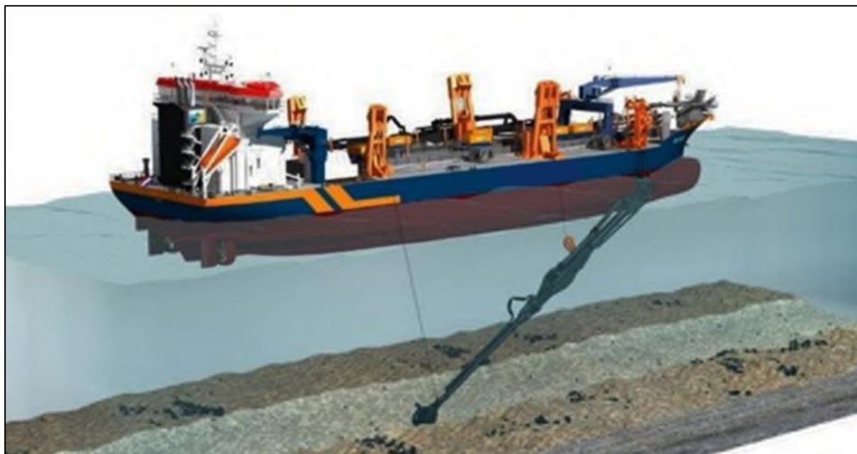
Figure 52: Representation of a trailing suction hopper dredger in operation with the arm deployed.
