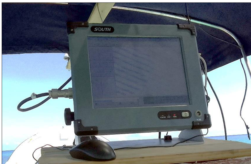
Photo 2: SDE-28S Echosounder, installed in the boat used to carry out the bathymetric survey.
