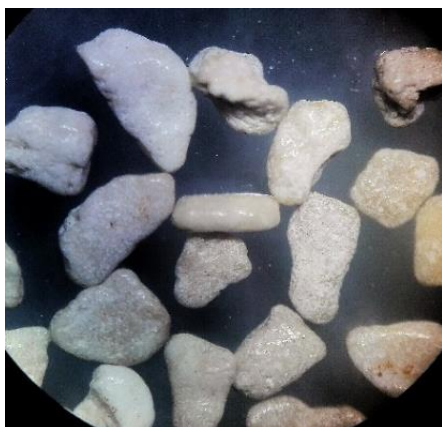
Photo 14: Grains of biogenic sand under the microscope. Sample taken at Runaway Bay. Skeletal remains of Halimeda algae.
